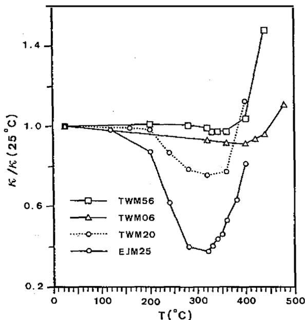
Fig. 9 Variations of normalized bulk magnetic susceptibility on heating for magnetite-, pyrrhotite- and greigite-bearing specimens. Symbols are the same as Fig. 2.
