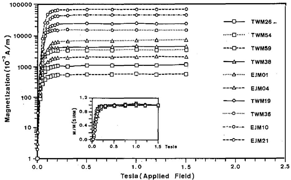
Fig. 2 Representative diagrams of acquisition of IRM for magnetite-, pyrrhotite- and greigite-bearing specimens, with symbol squares, triangles and circles, respectively. All of the SIRM are obtained below 0.2 Tesla in spite of different magnetic mineral constituent in the rocks. The inset shows their normalized IRM acquisition curves.
