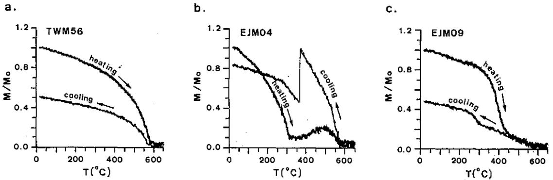
Fig. 7 Thermomagnetic curves of magnetite (a), pyrrhotite (b) and greigite (c) in a nitrogen atmosphere with a heating-cooling rate  $20^{\circ}\text{C}/\text{minute}$ . Magnetizations ( $M$ ) were normalized by dividing the initial value ( $M_0$ , room temperature). In Figure 7b, the interruption of cooling curve at  $370^{\circ}\text{C}$  is due to a man-made break of applied field to avoid an over-scale of increasing magnetization.
