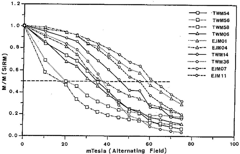
Fig. 5 Typical normalized alternating field (a.f.) demagnetizing curves of SIRM for magnetite-, pyrrhotite- and greigite-bearing specimens. Symbols are the same as Fig. 2.  $MDF_{SIRM}$  is the field strength which is required to eliminate one-half of SIRM.
