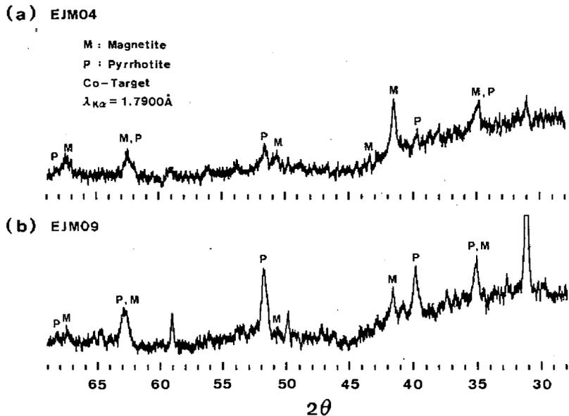
Fig. 8 X-ray diffraction spectra, revealing that after the first cycle run of thermomagnetic analysis, most of pyrrhotite has been transformed to magnetite (a), and greigite to pyrrhotite and magnetite (b). The original pyrrhotite and greigite X-ray diffraction patterns before thermal treatment had been shown in the previous study (Hornig *et al.*, 1992).
