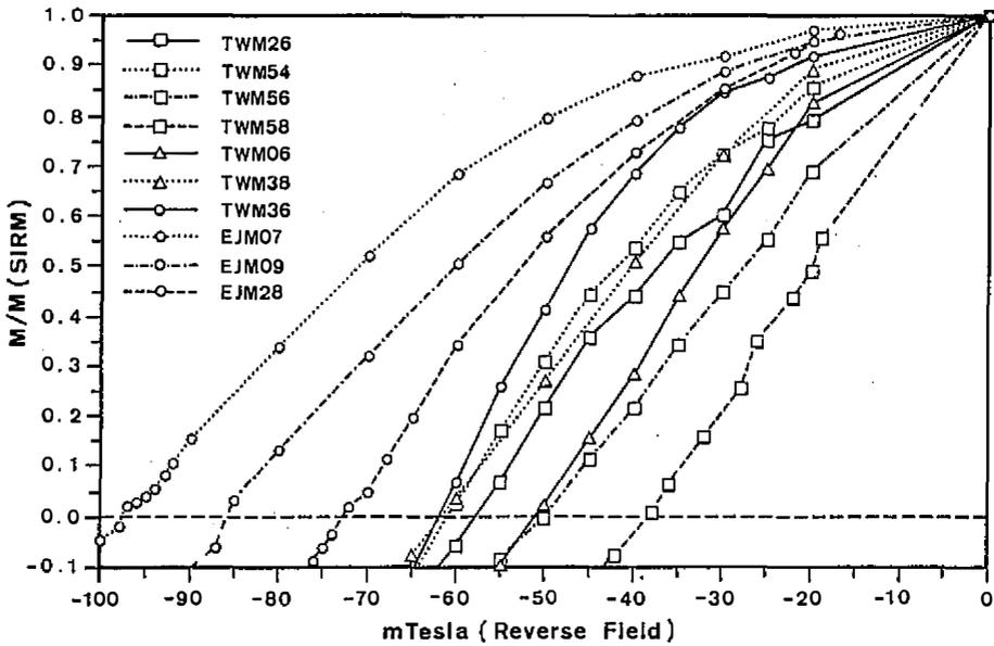
Fig. 4 Typical coercivity plots of SIRM versus reverse applied field for magnetite-, pyrrhotite- and greigite-bearing specimens. Symbols are the same as Fig. 2. Their coercivity forces ( $H_{cr}$ ) can be determined when magnetizations reduce to zero.
