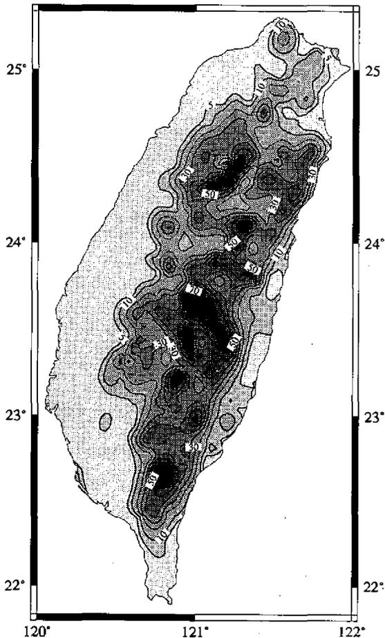
Fig. 5. Contour map of gravity terrain corrections in Taiwan. Contour interval: 5 mgal (correction  $\leq$  10 mgal), Contour interval: 10 mgal (correction  $>$  10 mgal)
