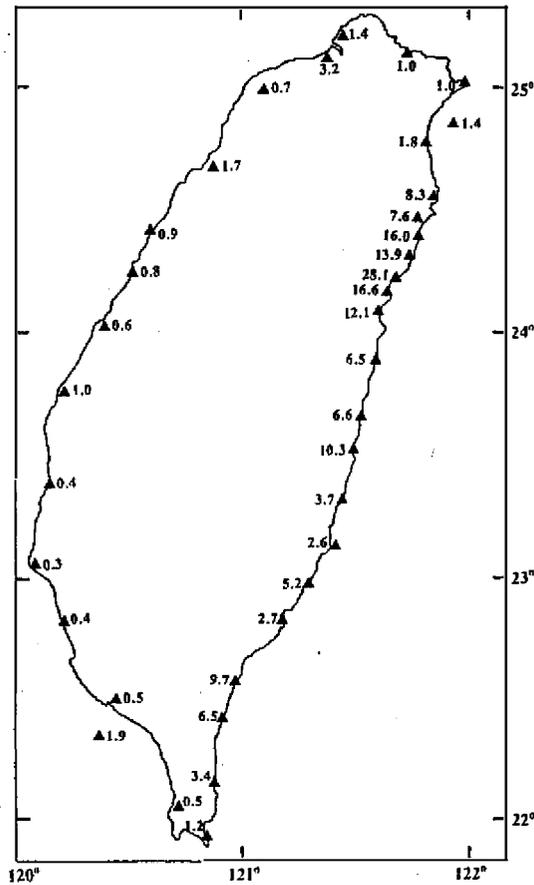
Fig. 8. Terrain corrections at stations along the coasts and offshore islands of Taiwan.
