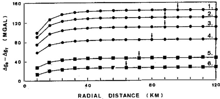
Fig. 4. Differences between Bouguer and terrain corrections( $\Delta g_B - \Delta g_T$ ) versus the radial distances for the representative stations. (■:Benchmark, ●:Triangulation point; 1.Taoshan: 3315m, 2.Yuantochieshan: 2888m, 3.Tochiatunshan: 2703m, 4. Chililoushan: 2492m, 5.Suyuan yakou: 1949 m, 6.Hsiangkuchia: 1781m)
