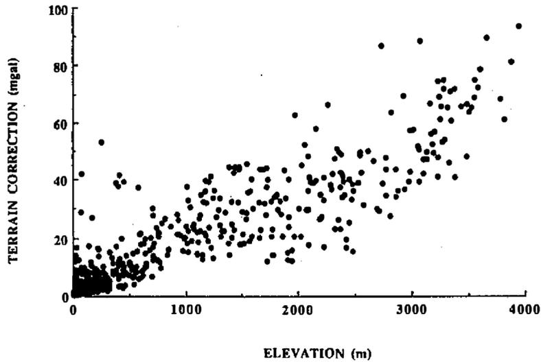
Fig. 6. Plot of terrain corrections with respect to station elevations.
