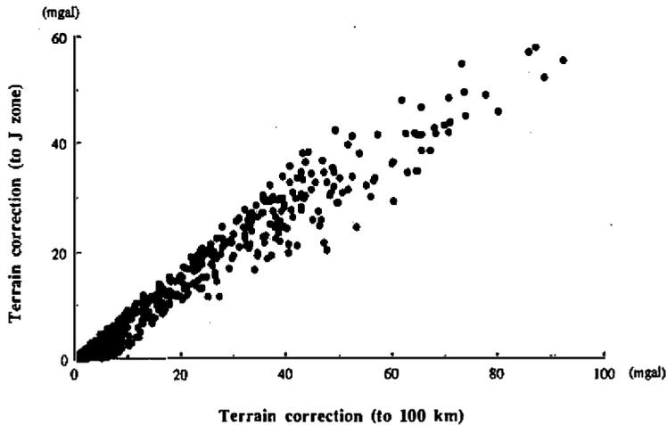
Fig. 7. Relationship between the corrections done to the distance of 6.5 km (to the Hammer J zone) and to the distance of 100 km.
