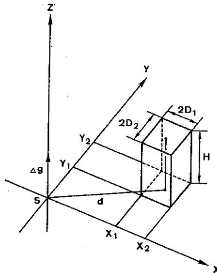
Fig. 3. Geometric relation between a gravity station S and a terrain prism with rectangular basis or the approximated line mass.
