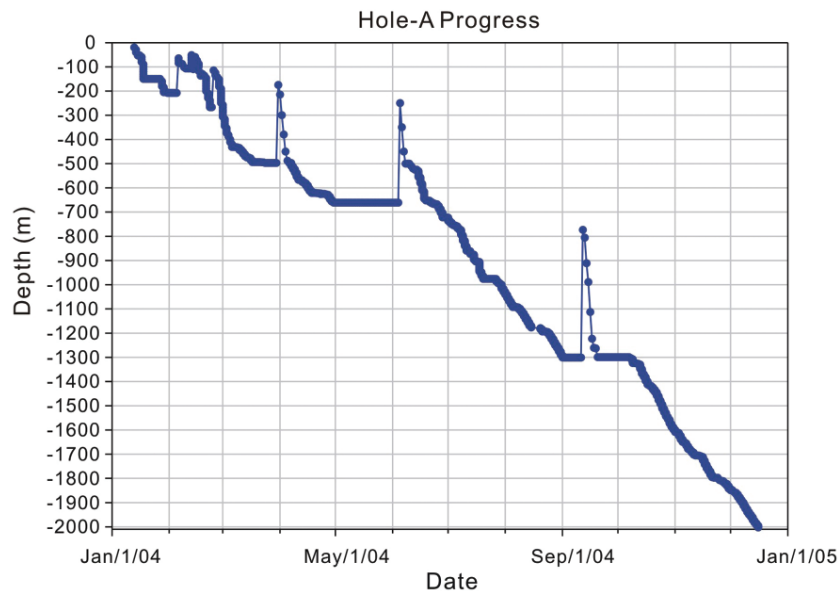
Fig. 2. Progress of Hole-A TCDP. Several long delays in the depths of 43 - 48, 140 - 150, 390, 661, and 1310 m were encountered by difficult geologic conditions, mechanical problems and standby time of logging.
